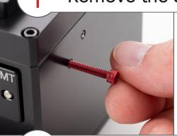
Re-install shipping screw if shipping or transporting the fibersect. Hand-tighten only.
