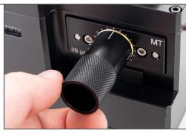
Adjusting Ring clockwise to cut closer to the ferrule face, counterclockwise to cut further away. Each calibration mark on the Adjusting Ring represents a 25 µm distance. The cut distance can be set between calibration marks for an even finer adjustment.
