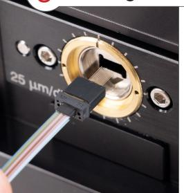
Hold the epoxied ferrule or connector at its base and carefully insert it into the Adapter Hole as far as it will go. For MT ferrules, the epoxy fill window must face down.
