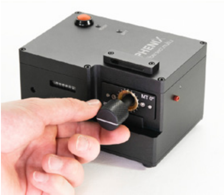
Adjusting the Slot Horizontally with Orientation Adjust Tool
