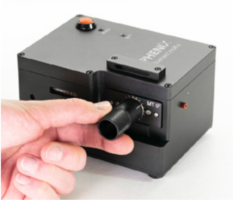
Adjusting Cut Length with Ring Adjust Tool
